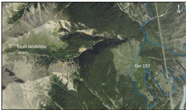
Figure 8. Example of evidence for recent landslide activity within the basin of Fan No. 197.
