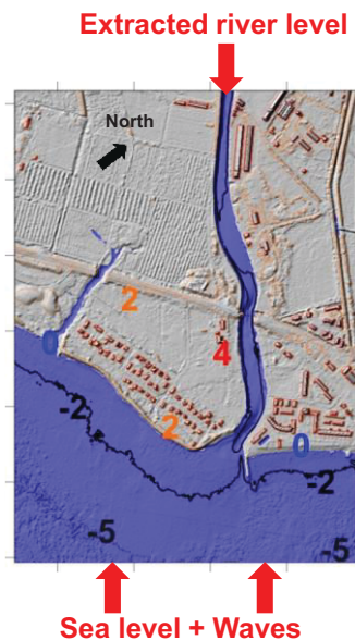
Figure 12. Forcing imposed to the finer grid on the hamlet of Cabanes du Gapeau.
