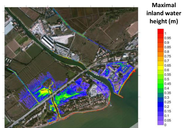
Figure 16. Maximal simulated water heights inland in the hamlet of Cabanes du Gapeau for a return period of 30 years at 2030 deadline.
