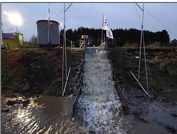
Figure 6. Observed aerated flow during the overflow experiment
