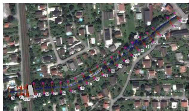
Figure 8. HEC Ras model of the Sierroz River between the Red bridge (right end) and the railway bridge (left end).
