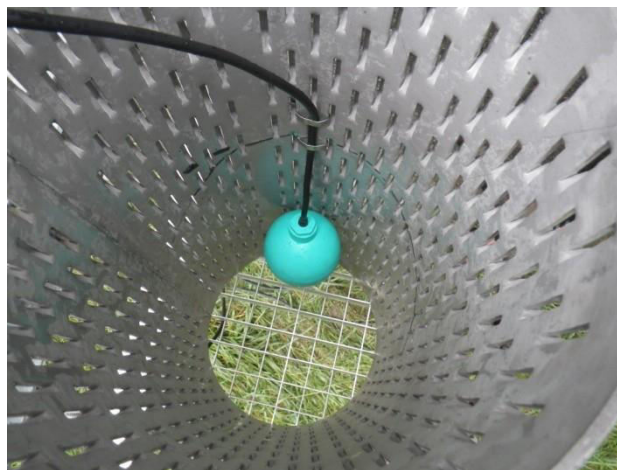
Figure 12. Zoom on the gauge for river level N1 detection
