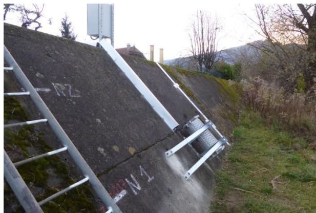
Figure 11. Automatic system of river level N1 detection
