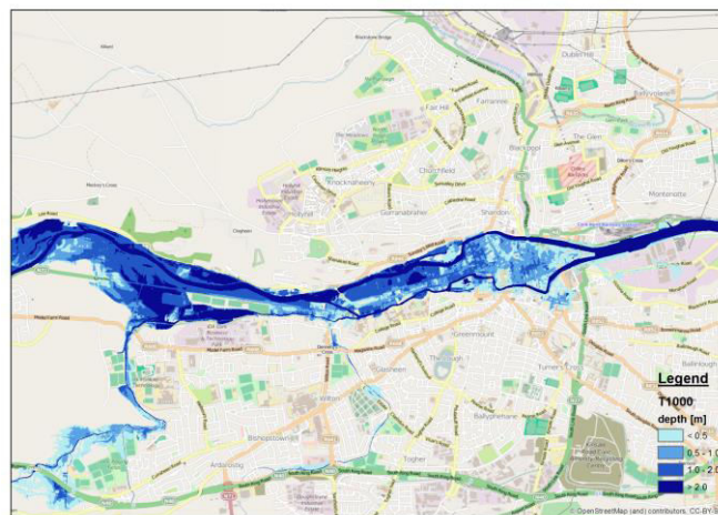
Figure 6. Flood map of the 1/1000 year flooding near Cork (based on the CFRAM Lee Pilot [13])
