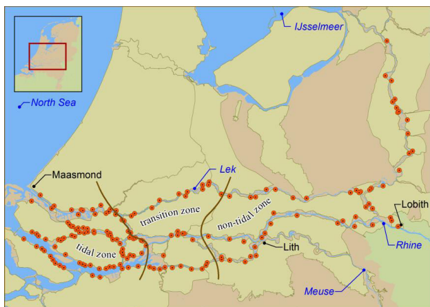
Figure 1. Map of the case study areas with the boundaries of the studied area (Lobith, Lith, IJsselmeer, North Sea), the three zones dominated by different flood types (tidal zone, non-tidal zone and transition zone), and the potential breach locations (red dots) (source: [3]).
