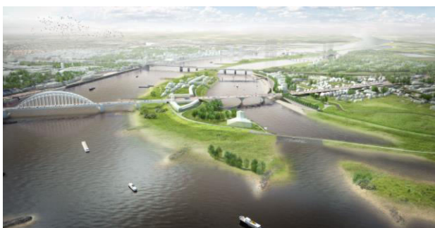
Figure 2. Drawing of the proposed creation of a discharge canal in order to broaden the river in Nijmegen (before and after) (Nijmegen City).
