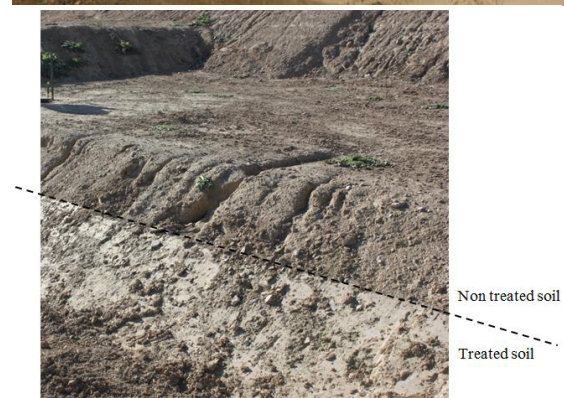
Figure 5. ABOVE : Non treated soil (Zone I) at left hand side, with erosion channels ; lime treated soil (Zone II) at right hand side, with no erosion channel.
