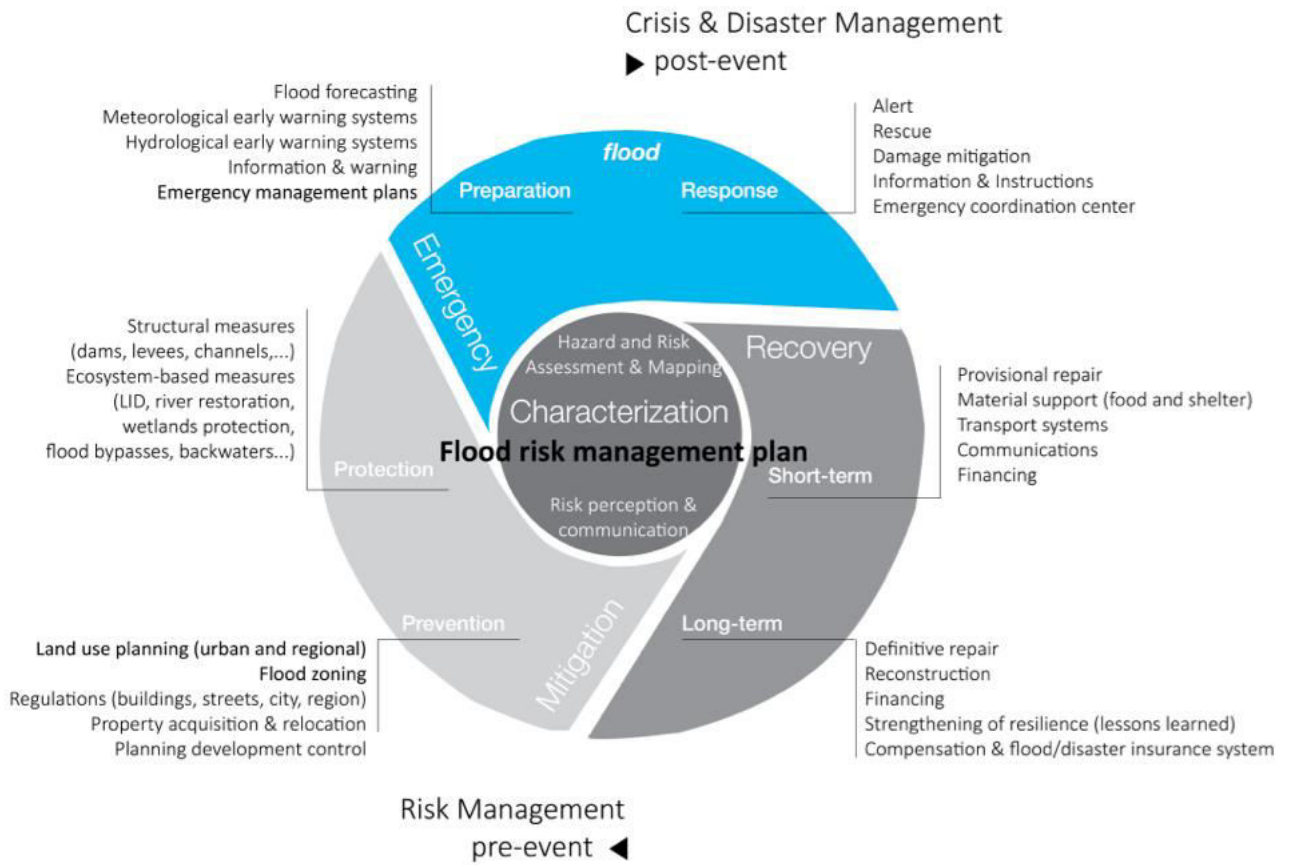
Figure 1. The flood risk management cycle (6).
