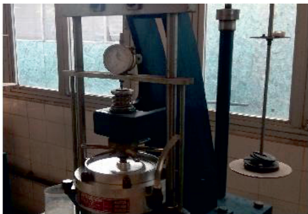
Figure 2. Swell Pressure Test.
