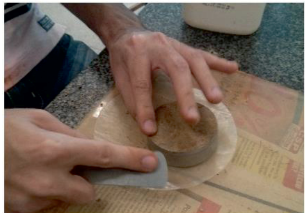
Figure 1. Moulding of specimens for Free Swell and Swell Pressure tests.
