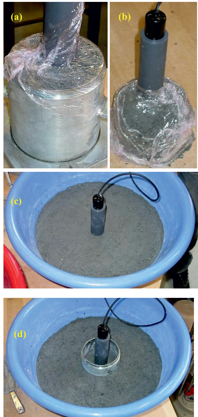
Figure 4. Samples of compacted Skiros weathered serpentinite with the ML-2x probe inserted for volumetric water content measurement a) still in the Proctor test compaction mould, b) after extrusion, c) of larger diameter, and d) of larger diameter but with the mould placed too.
