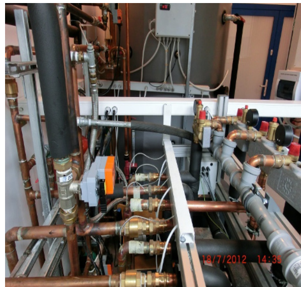
Figure 7. Pipe connections to the HT sorption refrigeration cycle, with thermometers and flow meters.
