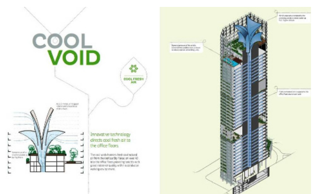
Figure 4. CapitaGreen (2012-2014), Architect Toyo Ito & Associates Architects. Scheme air flow throughout the building, effectively regulating the building's temperature (source : [8]).
