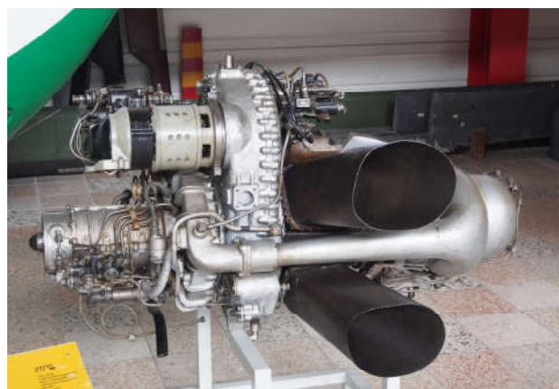
Figure 7. GTD-350 engine overview.
