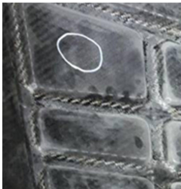
Fig. 7. CFRP stiffened aerospace panel with teflon insert (diameter 30 mm)
