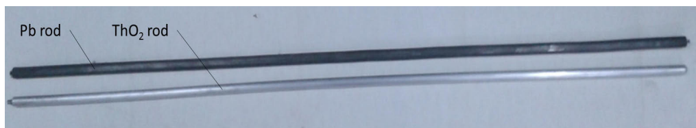
Fig. 2. Pb and ThO 2 rods.
