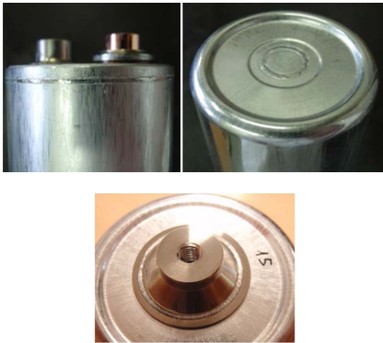
Figure 2. VL51ES Li-ion cell mechanical envelop
