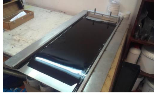
Figure 1. Stabilized casting process for buckyfilms production
