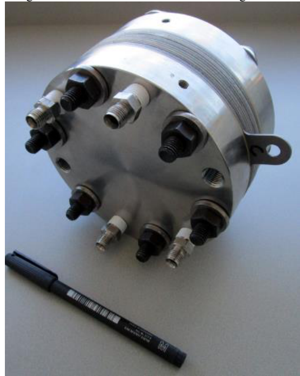
Figure 7 1kW 100 bar PEM electrolyser with mass optimised cell plates, but with non-optimised endplates
