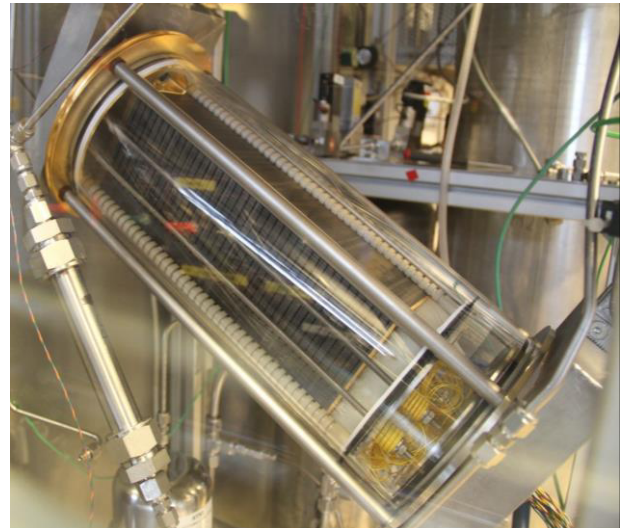
Figure 2 HTPEM FC stack used in testing of the closed loop RFCS breadboard demonstrator in 2012 [6] (here without thermal insulation)
