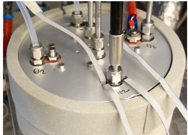
Figure 4 Full size short stack installed into the test stand and ready for testing
