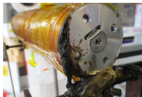
Figure 11 – VES140 cell sample after the ARC test with the positive side opened
