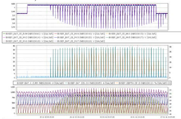
Figure 4. IOV FM02 battery cycling during eclipse season 9
