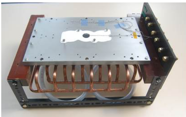
Figure 2. Regulated Baseplate with thermocouple and CHO-THERM under Cell-Package
