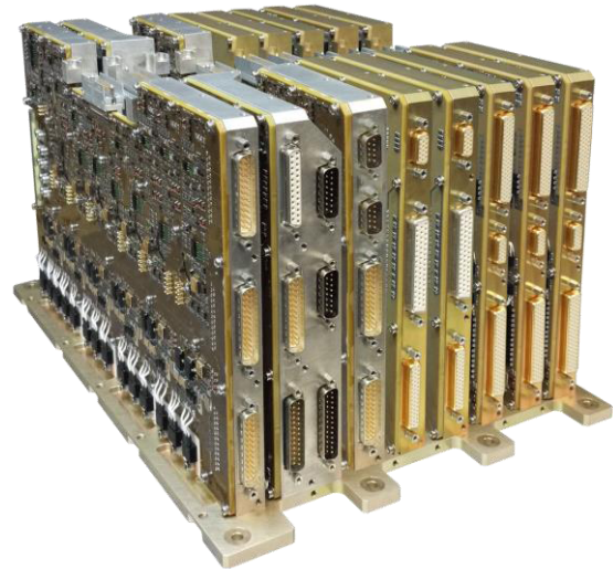
Figure 1. LEO PCDU EVO EM during integration in the configuration for Merlyn mission
