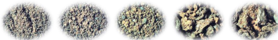
Fig. 5. Fine-grained recycling aggregate with fraction division. From left 0/0.063; 0.125/0.25; 0.25/0.5; 0.5/1; 1/2.
