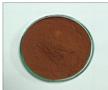
Fig. 3. Slag from the combustion of municipal sewage sludge, fraction < 500 µm.
