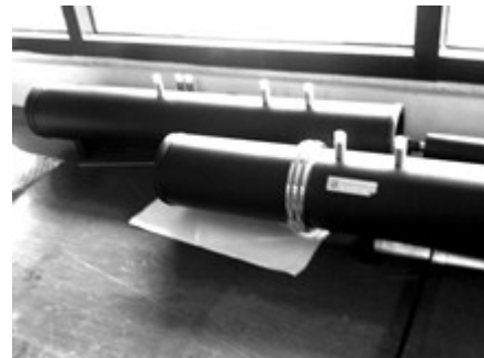
Fig.2. The Impedance Tube with microphones
