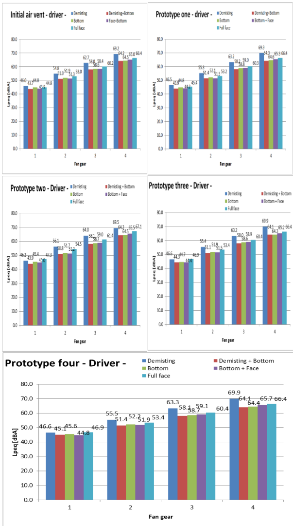
Fig. 6. Sound pressure level for driver position with different air vents
