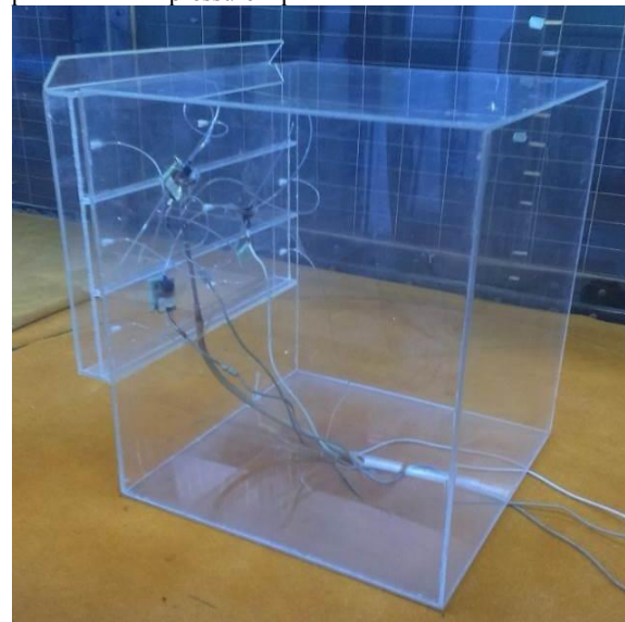
Fig. 4. Front view of the building model inside the wind tunnel – position of the pressure taps.
