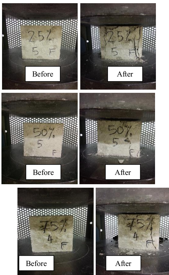
Fig. 1. The crack behaviour before and after compression test for all proportion.
