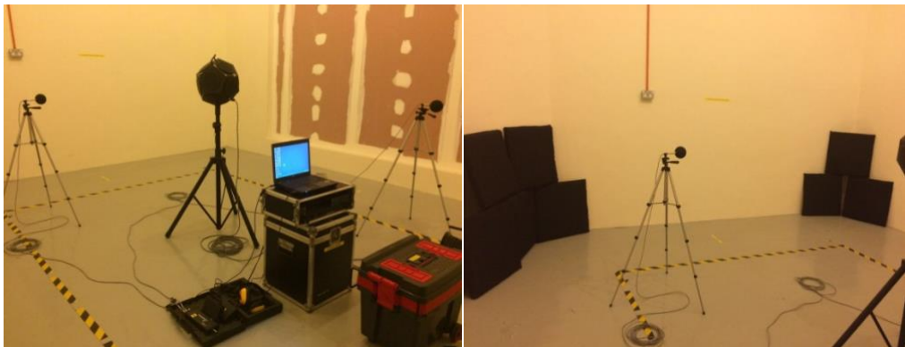
Fig. 4. Equipment setup and layout of the echo chamber.
