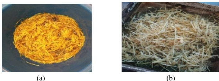
Fig 3. Bagasse fibre after treated in solution after 1 hour (a) 5% NaOH treated, (b) 5% HCL treated.
