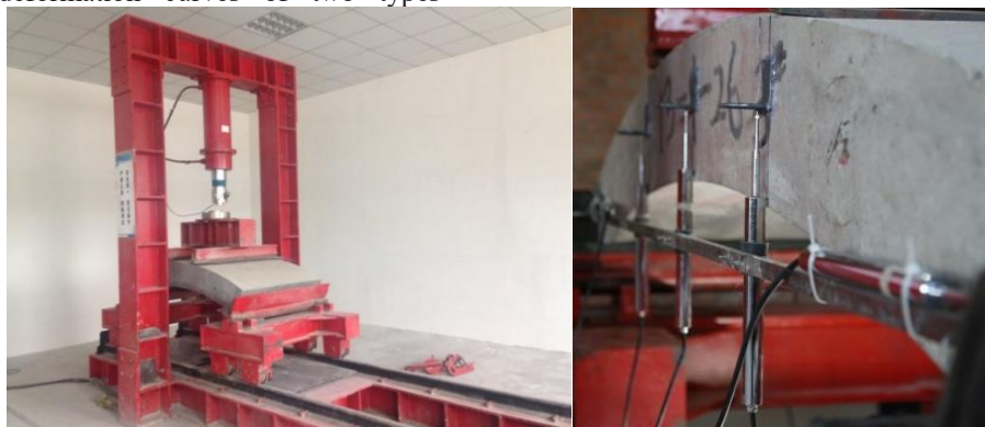
Figure 3 The segment flexural testing setup
