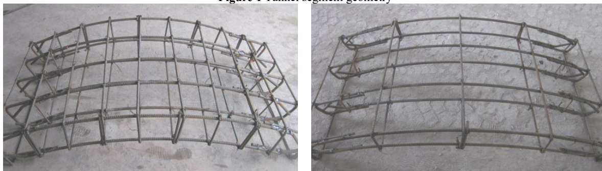
Figure 2 The rebar cage of segments (Left: RC segment; Right: UHPFRC segment)
