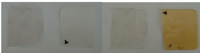
Fig. 9. Reference sample TOPAS and sample after 1120h weathering ageing (1) and reference sample TOPAS (1) and sample after 1120h UV ageing (2).
