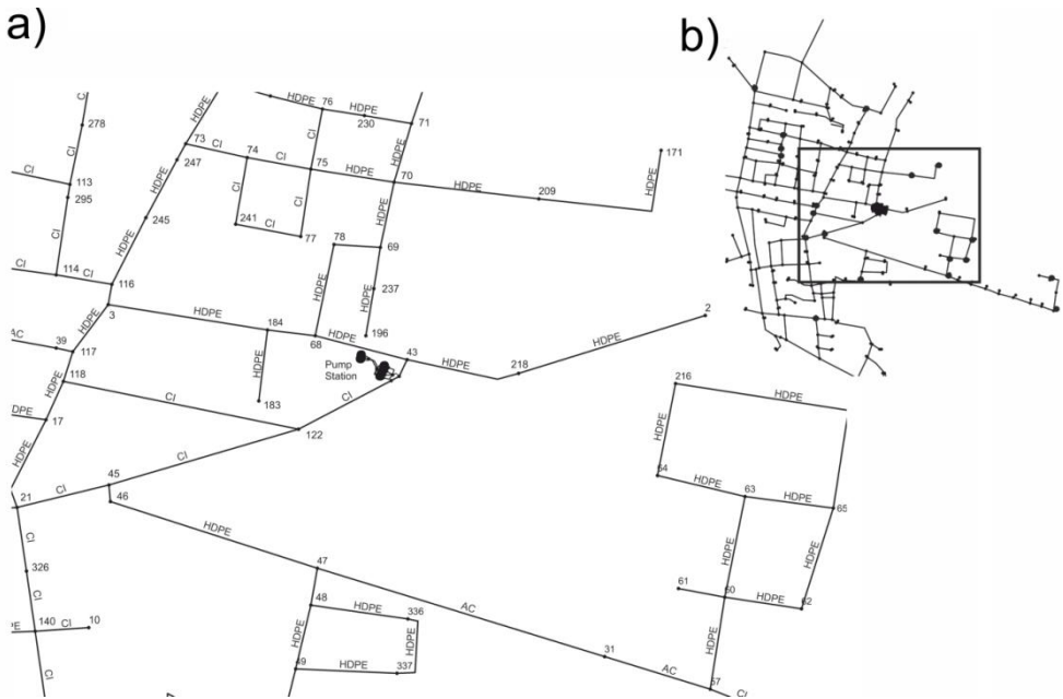
Fig. 1. The selected portion of the water supply network Poddebice, pipe material: plastic - HDPE; asbestos cement - AC; cast iron - CI (a); scheme of the water supply system Poddebice with the marked locations of the hydrant fire flow demand (b).
