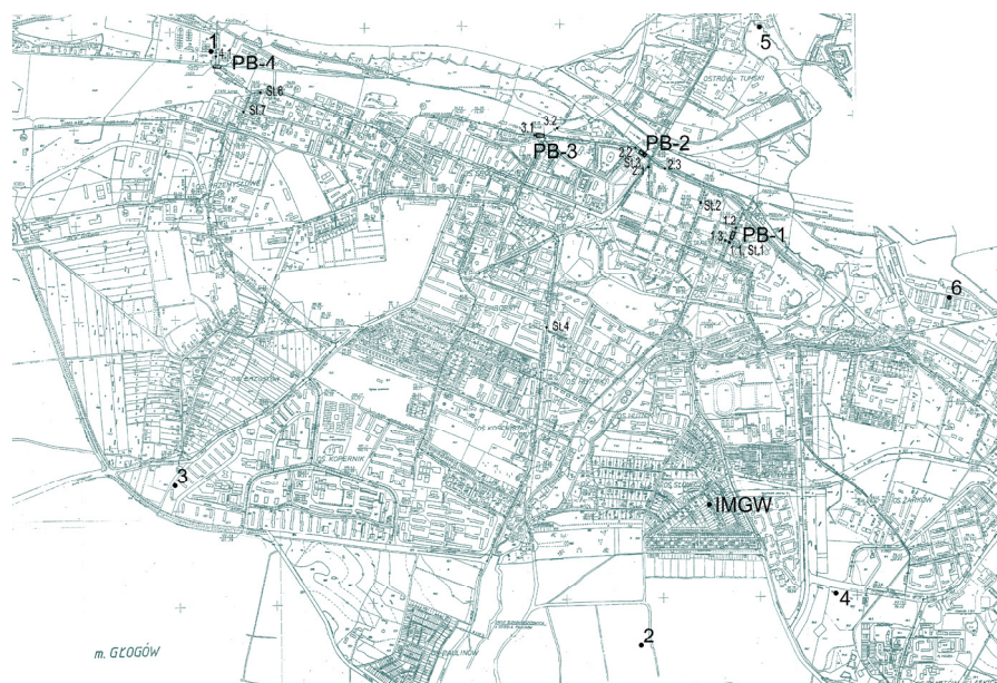
Fig. 1. Location of rain gauges and measurement stations in the area of the city: PB-1–4 - overflow structures; St.1–7 - measurement stations in the period 1998–2000; IMGW - weather station in the period 1998–2000; 1.1–4.1 - measurement stations in the period 2011–2014; 1–6 - rain gauge in the period 2011–2014 [1, 2].
