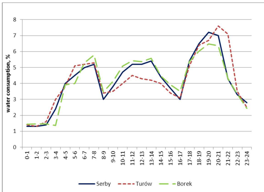
Fig. 4. Hourly distribution of water consumption in systems supplying villages.
