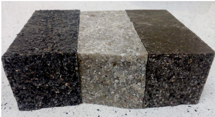
Fig. 4. Photograph of breakthroughs of mortar samples containing 50% modifier, created after the flexural strength test.
