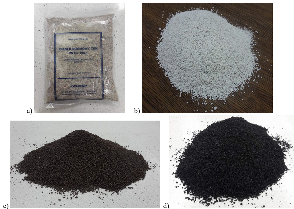
Fig. 2. Aggregates used in the preparation of mortar samples a) perlite, b) expanded clay, c) rubber waste, d) standard sand.
