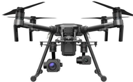
Fig. 3. UAV of DJI Matrice 210 type proposed for IR thermography examination [16].
