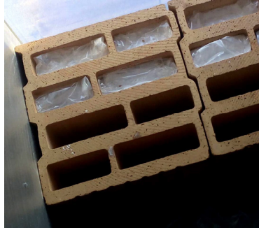
Fig. 3. Ceramic block with two slots filled with PCM.
