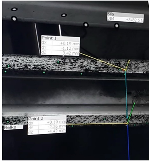
Fig. 6. Representation of displacement measurement in the GOM Correlate.
