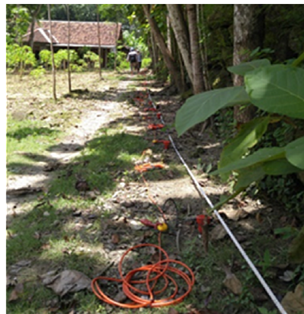
Fig. 4. Example of the geophone configuration.
