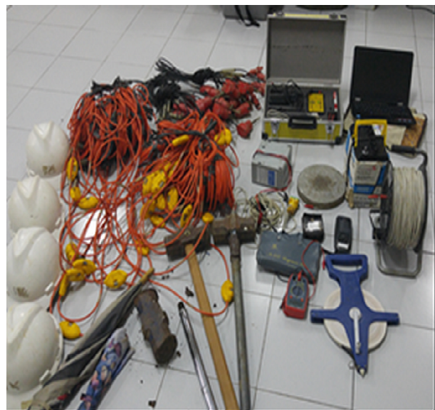
Fig. 3. Equipment of MASW method.
