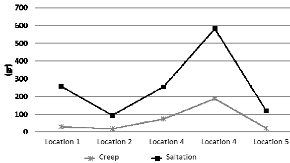
Fig. 5. Comparison of sand movement weight trapped on sand sampler. Saltation sand is bigger than creeping sand.
