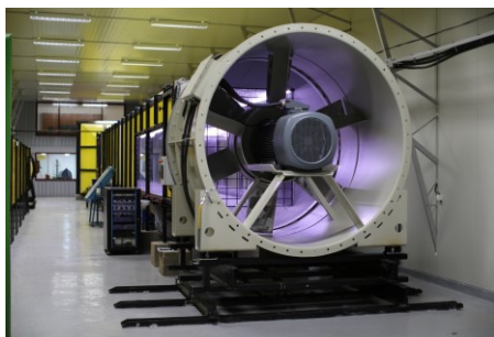
Fig. 2. The new refurbished boundary layer wind tunnel TASL1-M [4-5].
