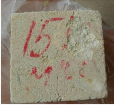
Fig. 5. Cracks on the untreated sample treatment.
