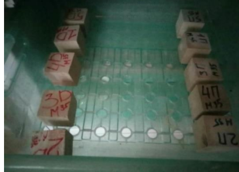
Fig. 4. Thawing in vessels with water.
