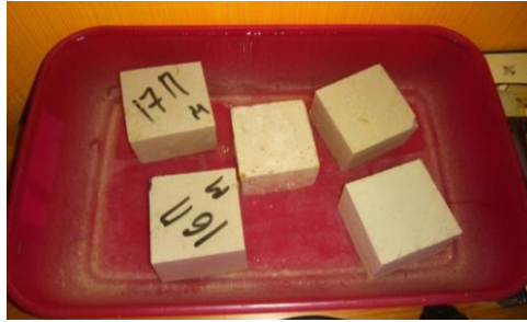
Fig. 2. Samples immersed in a vessel with water.
