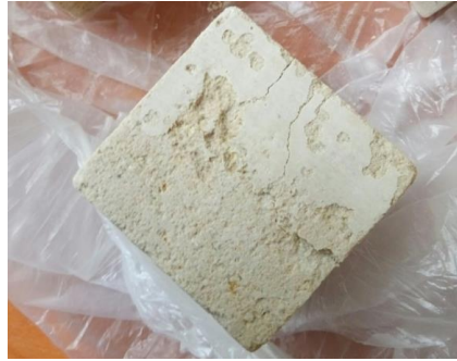
Fig. 6. Cracks and peelings on the untreated sample.
