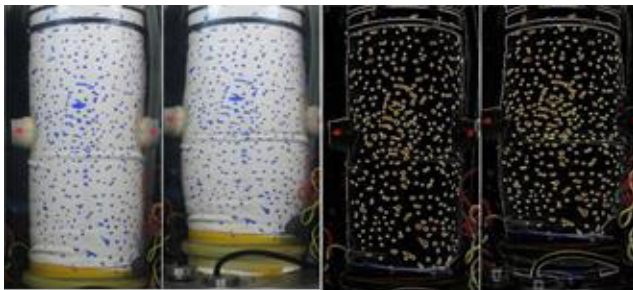
Fig. 11. Locating the boarder of specimens during shearing
