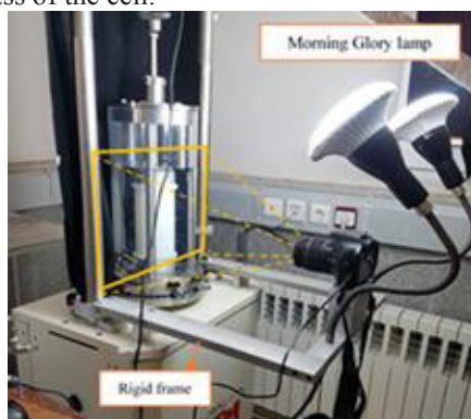
Fig. 1. Image processing frame and two morning glory lamps
