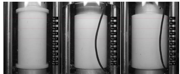
Fig. 2. Placement of cylindrical dummies for considering magnification and distortion effects
