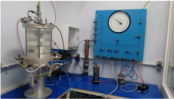
Fig. 1. View of the Bishop-Wesley triaxial cell
