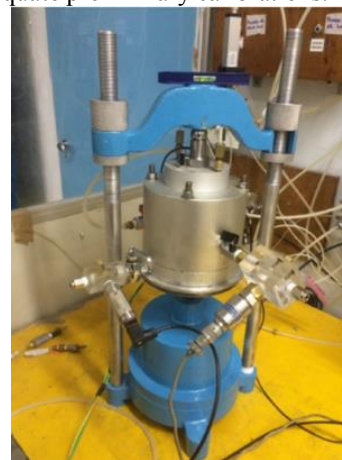
Fig. 2. View of the suction controlled K_0 cell with the self-supporting loading frame
