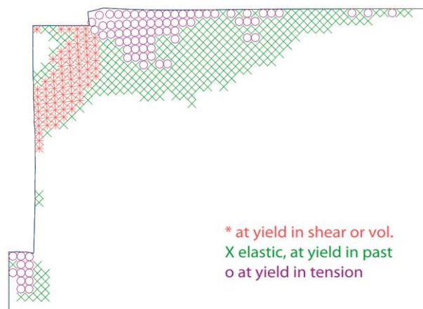
Fig. 10. Yielding state of the surrounding clay at the final step of loading for ordinary stone column
