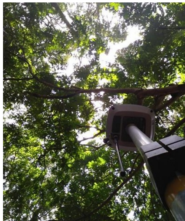
Fig.4. Illustration of satellite obstruction in the field due to forest canopy. The obstruction can be up to 90 percent.
