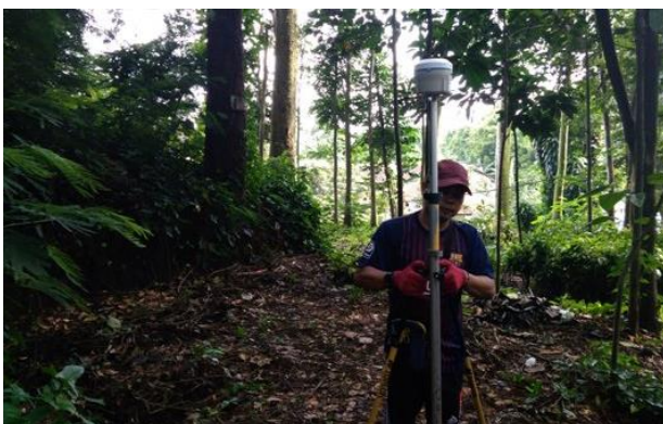
Fig.6. Documentation of RTK Multi GNSS in National Forest Park in northern of Bandung
