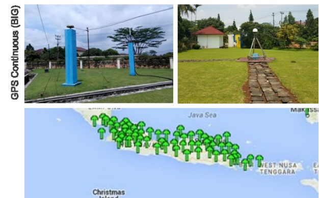
Fig.5. Documentation of Benchmark of CORS BIG and map of all location of Benchmark around Java Island.
