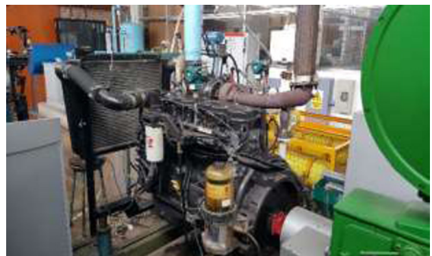
Fig 1. Main Diesel Motor for experimental tests, Energy Laboratory of Pontificia Universidad Católica del Perú
