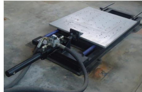
Fig 6. Uniaxial seismic shake table at UIS.
